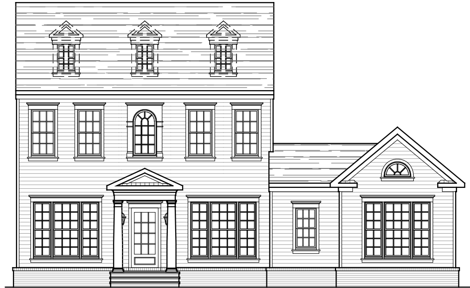
FRONT ELEVATION STANDARD ELEVATION 3A STANDARD 9'-0" CEILING 02-07-2025
