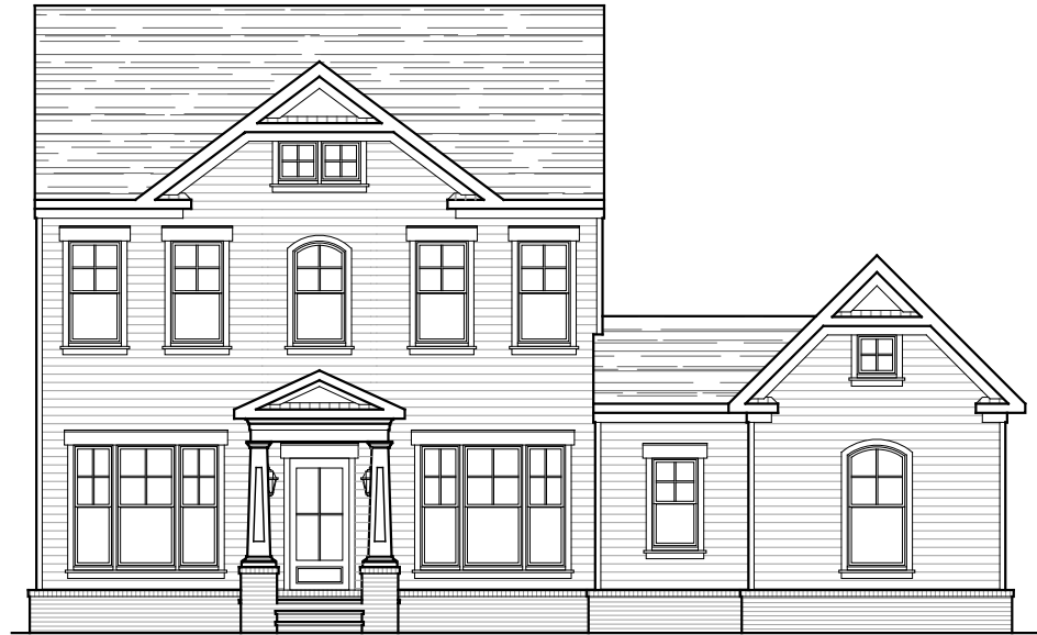
FRONT ELEVATION STANDARD ELEVATION 5A STANDARD 9'-0" CEILING 02-07-2025
