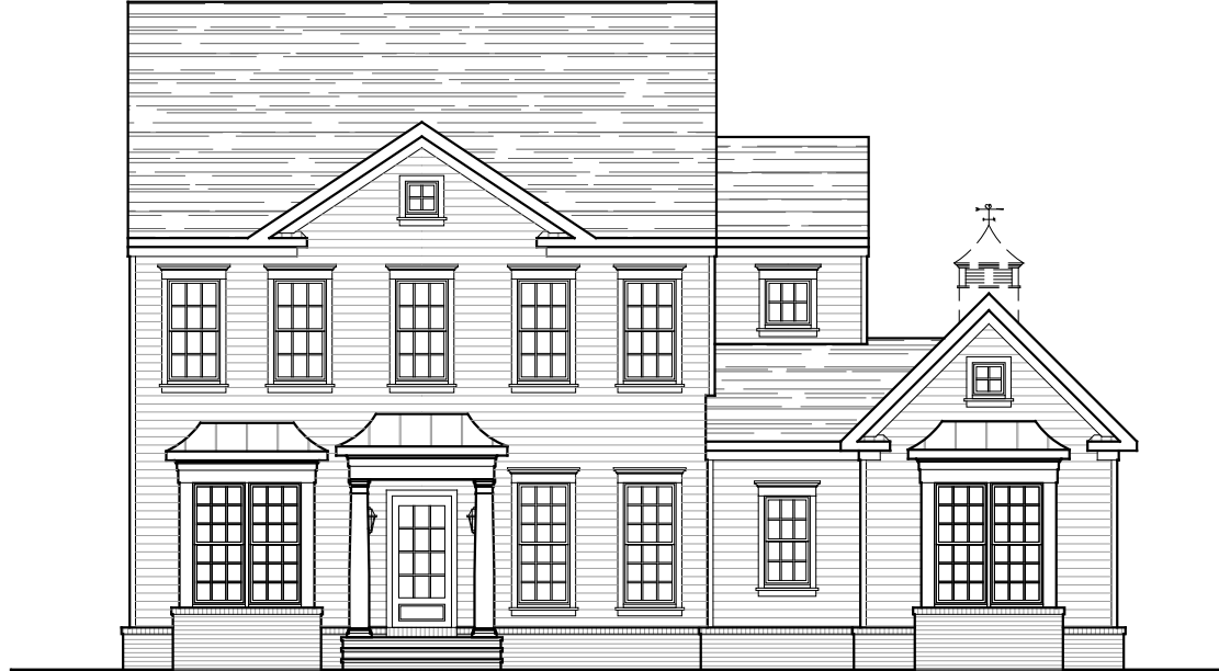
FRONT ELEVATION STANDARD ELEVATION 8A STANDARD 9'-0" CEILING 08-08-2025
