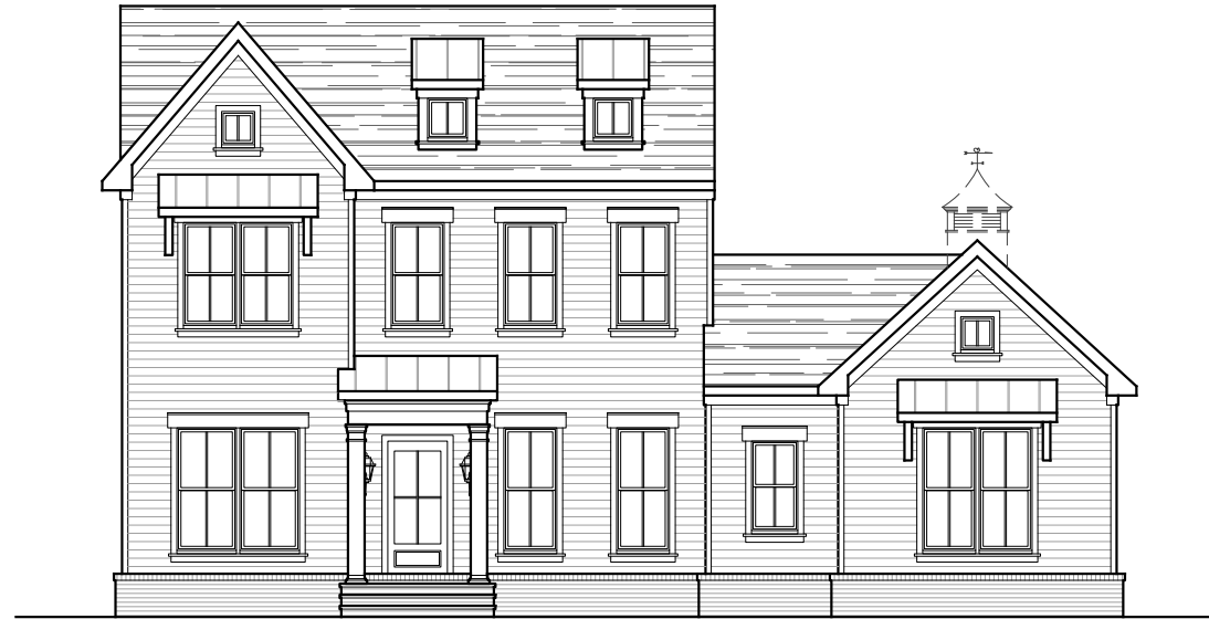
FRONT ELEVATION ELEVATION 5A STANDARD 9'-0" CEILING 01-22-2025
