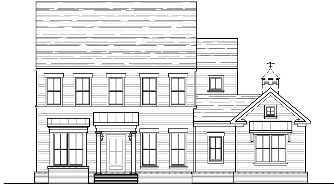
FRONT ELEVATION STANDARD ELEVATION 3A STANDARD 9'-0" CEILING 01-24-2025
