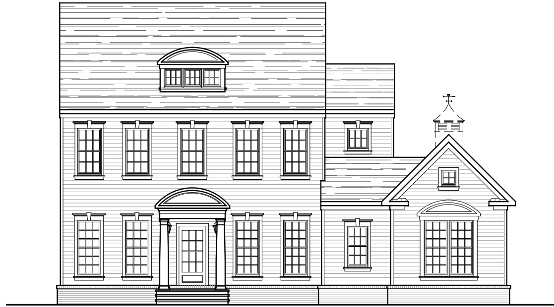
FRONT ELEVATION STANDARD ELEVATION 7A STANDARD 9'-0" CEILING 01-24-2025
