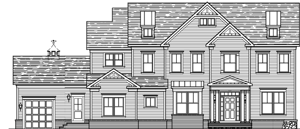
FRONT ELEVATION * ELEVATION #5A W/ FRONT LOAD 1-CAR GARAGE STONE IS OPTIONAL 12-16-24
