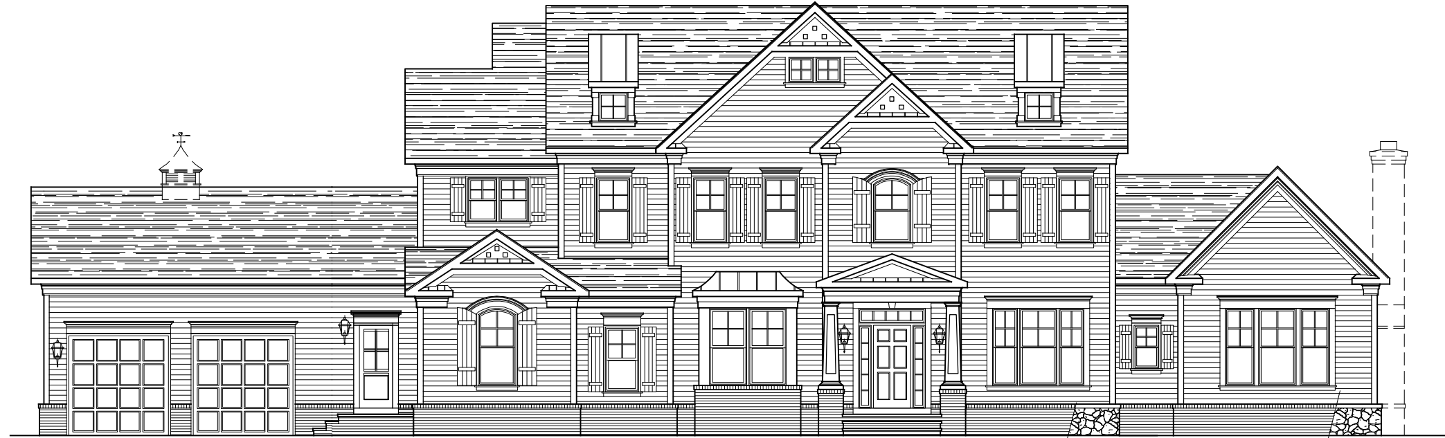
FRONT ELEVATION * ELEVATION #4A W/ FRONT LOAD 2-CAR GARAGE W/ CLUB ROOM STONE IS OPTIONAL 12-16-24
