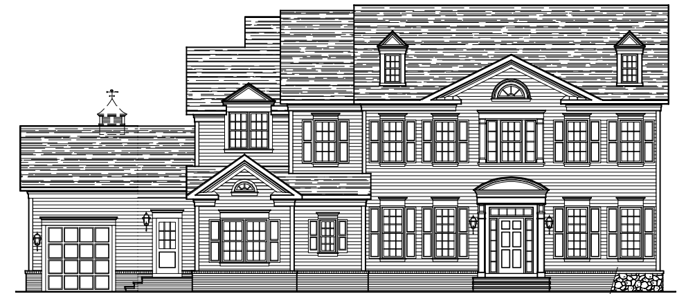
FRONT ELEVATION * ELEVATION #2A W/ FRONT LOAD 1-CAR GARAGE STONE IS OPTIONAL 12-16-24
