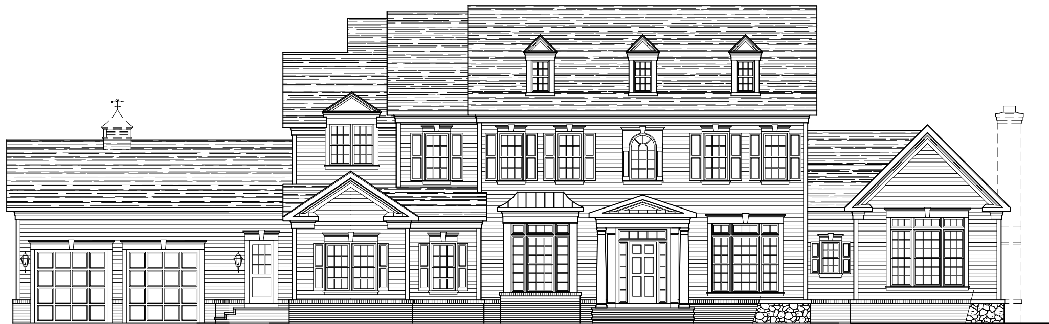
FRONT ELEVATION * ELEVATION #14A W/ FRONT LOAD 2-CAR GARAGE W/ CLUB ROOM STONE IS OPTIONAL 12-16-24
